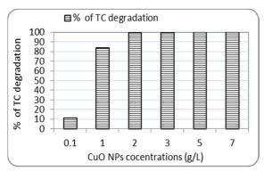
Figure 7: Effect of CuONPs different concentrations on TC bacterial degradation percentage.
