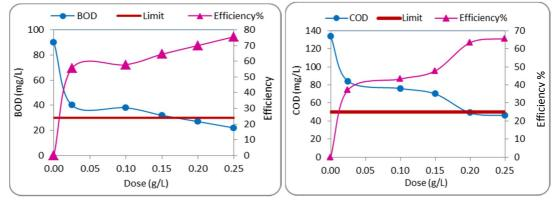
Figure 1: Variation of BOD and COD concentrations and their removal efficiencies with the dose of ALUM added to raw wastewater from El-Rahway drain (( $R^2 = 0.62$  and 0.79, respectively).
