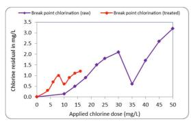
Figure 5: Residual chlorine versus applied chlorine dose for composite wastewater collected from El-Rahway drain and treated water samples by ALUM.
