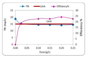
Figure 2: Effect of ALUM doses on total nitrogen (TN) concentration and removal efficiency ( $R^2$ = 0.69).
