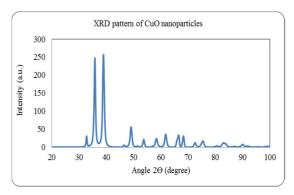
Figure 6: XRD pattern of prepared CuOnanoparticles by sol - gel method.
