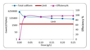
Figure 4: Variation of Total bacteria count (TBC) concentration and its removal efficiency with the dose of ALUM added to raw wastewater from El-Rahway drain ( $R^2$ = 0.47).
