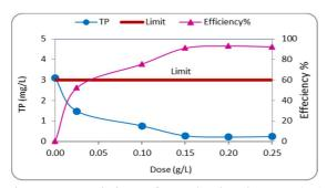
Figure 3: Variation of Total phosphorous (TP) concentration and its removal efficiency with the dose of ALUM ( $R^2$ = 0.73) added to raw wastewater from El-Rahway drain.
