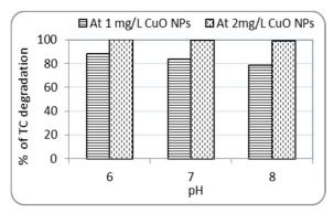
Figure 8: Antibacterial of CuO NPs on TC bacterial degradation percentage with different pH (6,7 and 8).
