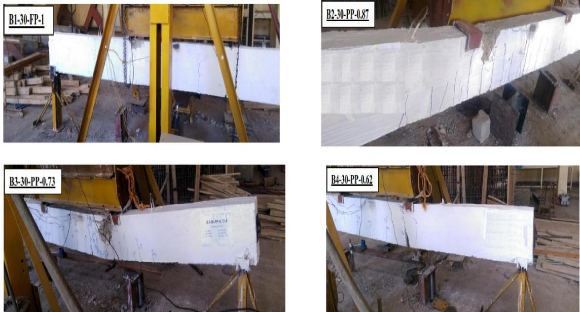
Fig. (6) Crack patterns at failure of all tested beams
