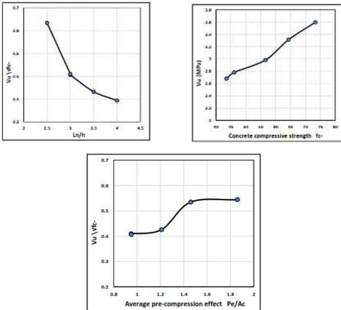
**Figure 6.** shear strength of tested beams
