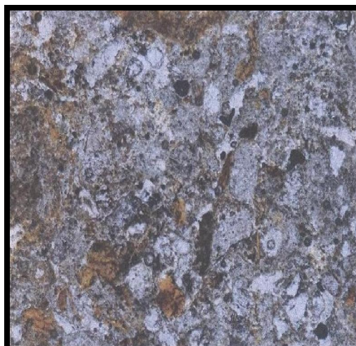
Fig. (6): Photomicrograph of Conglomerate sample.
