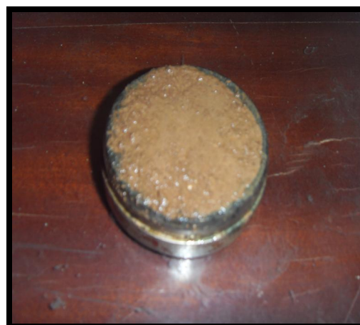
Fig. (2): Sample after trimmed in Oedometer cylinder
