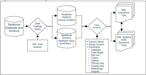
Figure 1. Architecture of converting a relational database into an XML document
