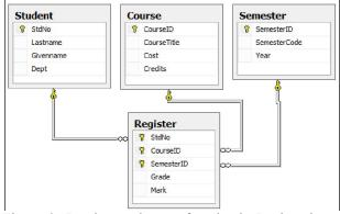
Figure 2. Database schema of a simple Registration Application
