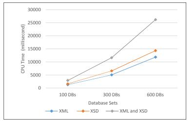
Figure 3. CPU time of generating XML document and XSD schema
