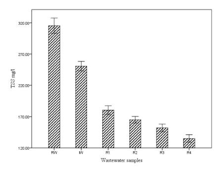
Figure 3. Reduction of total suspended solids of textile wastewater by gamma irradiation
