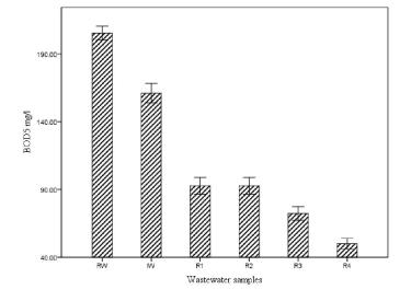
Figure 5. Reduction of BOD<sub>5</sub> of irradiated wastewater in presence of  $H_2O_2$
