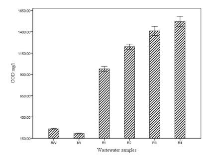
Figure 4. Variation of COD values of gamma irradiated textile wastewater in presence of  $H_2O_2$
