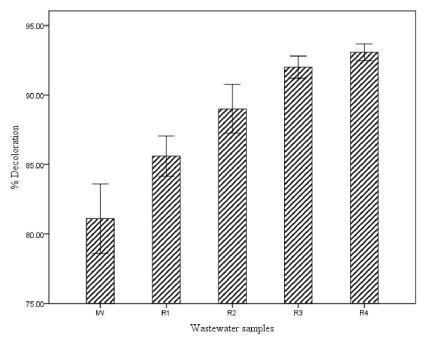
Figure 2. Color reduction (%) of wastewater in presence of H<sub>2</sub>O<sub>2</sub> after gamma irradiation
