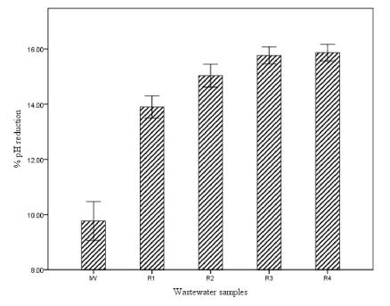
Figure 1. Reduction of pH of textile wastewater after gamma irradiation in presence of H<sub>2</sub>O<sub>2</sub>
