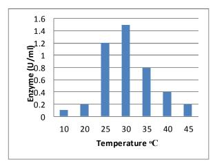
Fig. 2. Effect of different temperature on PHB degradation (enzyme production, U/ml) by the selected fungal isolate
