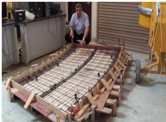
Picture 2: Adding reinforcement to the model without cross frames
