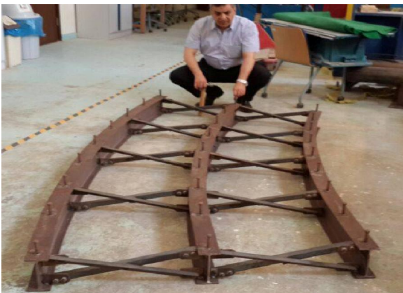
Picture 1: Assembly of the steel girders for the model with 3 cross frames
