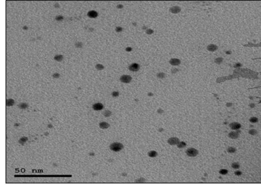
**Figure (5):** TEM image of silver nanoparticles (50 nm scale).
