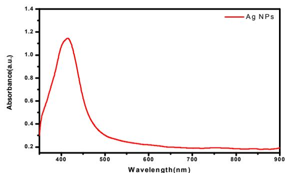
**Figure (3):** the absorption rate curve of silver nanoparticles solution
