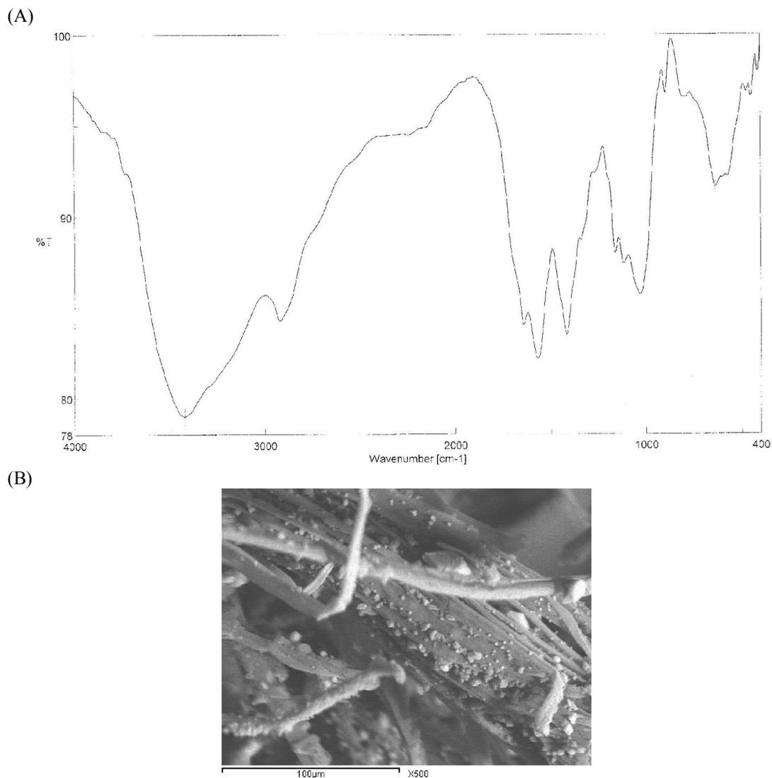
**Figure 2:** (A) FT-IR for methyl cellulose and (B) SEM for methyl cellulose
