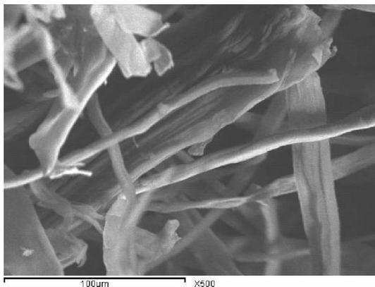
**Figure 1:** (A) FT-IR for bleached bagasse pulp and (B) SEM for bleached bagasse pulp
