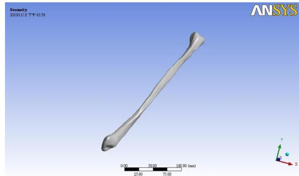
Figure 14. The original unreformed human fibula corresponded to the third mode shape.
