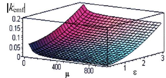
Figure 6 – The electric machines with the distributed secondary system external magnetic field coefficient module dependence from Reynolds magnetic number and from external magnetic conductor magnetic permeability
