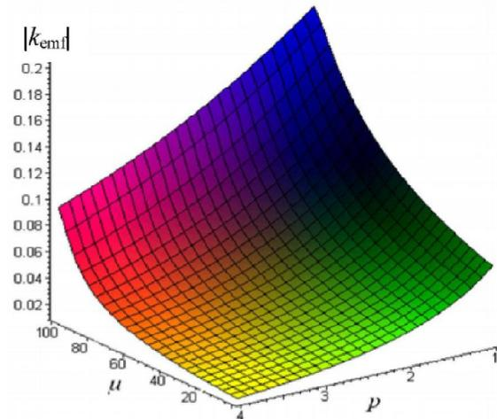
Figure 4 – Induction motor EMF coefficient dependence from number of pole couples
