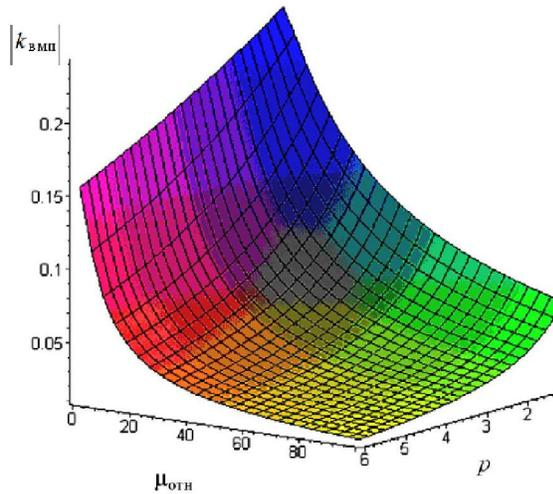
Figure 5 – Direct current electric machine external magnetic field coefficient module dependence from external magnetic conductor magnetic permeability and pole couples number
