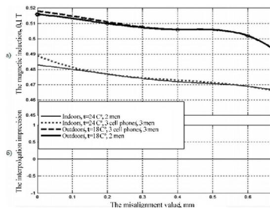
Figure 3 – The results of ACMB EMF measurements (the bowl thickness is 9 mm): a – the results of ACMB EMF as diagnostic criterion; b – the results of environment conditions influence on EMF parameters
