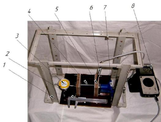
Figure 2 – The installation for carrying out the pilot studies of axial controlled magnetic bearing EMF as diagnostic criterion: 1 – the engine support; 2 – the calliper; 3 – the indicator of the hour type; 4 – the rod; 5 – the axial magnetic bearing; 6 – the Hall sensor; 7 – the pusher; 8 – the milliteslameter
