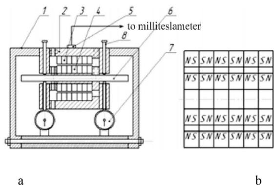
Figure 1 a –the experimental installation for EMF probes as diagnostic criterion of RCMB; 1 b – RCMB design: 1–engine support (bed); 2–controlled magnetic bearing; 3–external set of magnetic rings of NdFeBN33; 4–internal set of magnetic rings of NdFeB N33; 5–Hall sensor; 6–shaft; 7–indicator of the hour typ; 8–pusher
