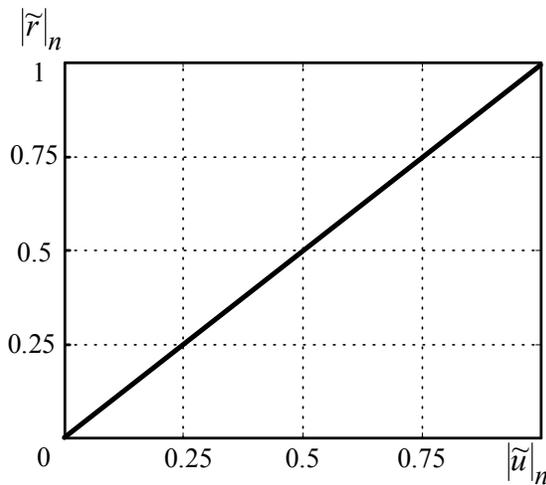
**Fig. 3 Normalized amplitude characteristic of the PA after its linearization with the help of DPGMP precompensator**
