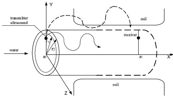
**Fig. 2.** Ultrasound extending inside an underground pipe
