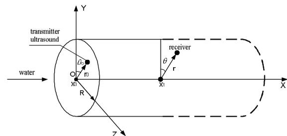
**Fig. 1.** Location of the ultrasound transmitter and receiver inside the pipe
