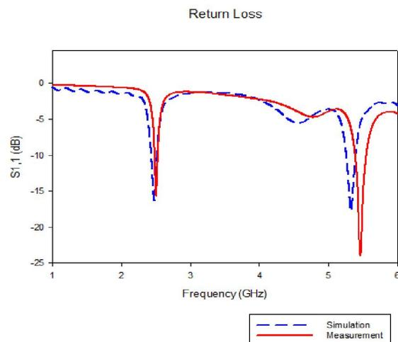
Figure 8. Simulated and Measured Return Loss
