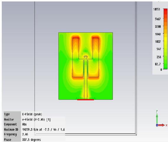
Figure 4. Current distribution at E-Field at 2.45 GHz
