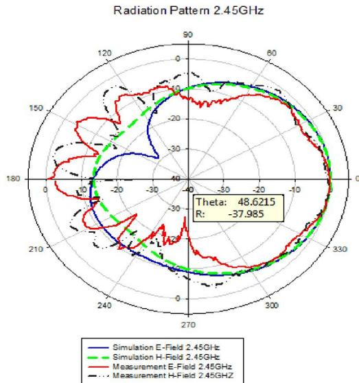
Figure 9. Simulated and Measured Radiation Pattern at 2.45 GHz.
