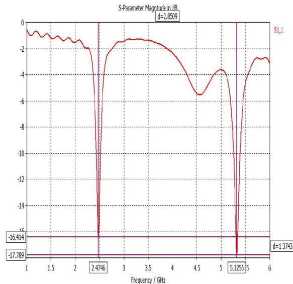
Figure 3. Simulated Return Loss
