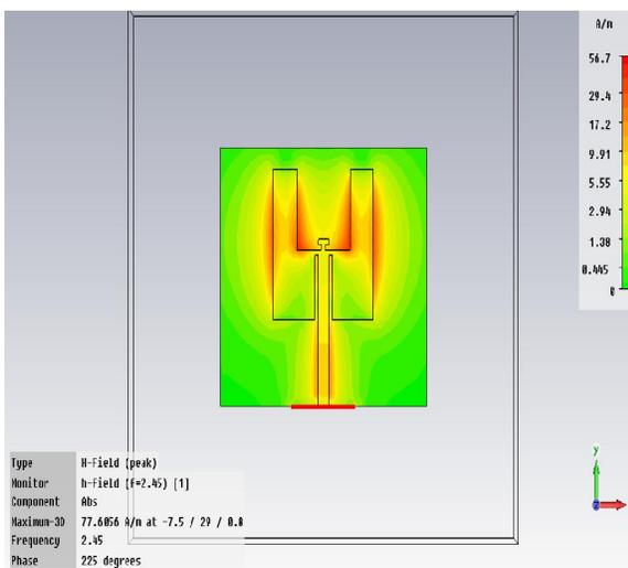
Figure 6. Current distribution at H-Field at 2.45 GHz
