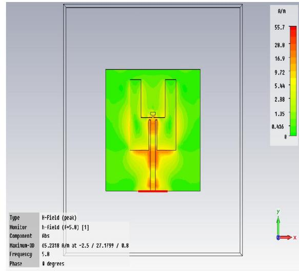
Figure 7. Current distribution at H-Field at 5.8 GHz
