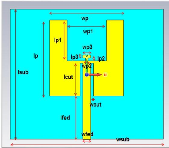
Figure 1. Front view of the proposed antenna structure
