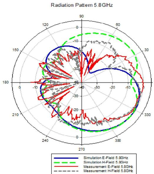
Figure 10. Simulated and Measured Radiation Pattern at 5.8 GHz.
