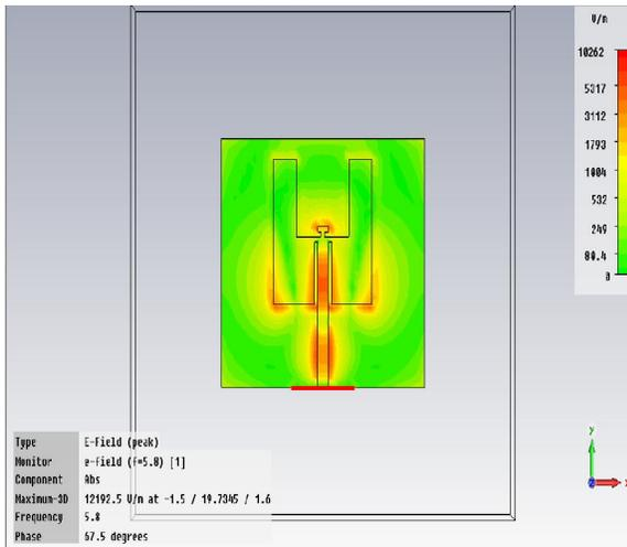
Figure 5. Current distribution at E-Field at 5.8 GHz
