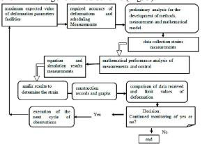
Figure 3. Schematic plan of monitoring and observation of deformation of engineering structures
