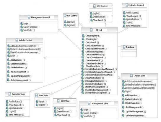
Figure 5: MVC diagram for OCMM
