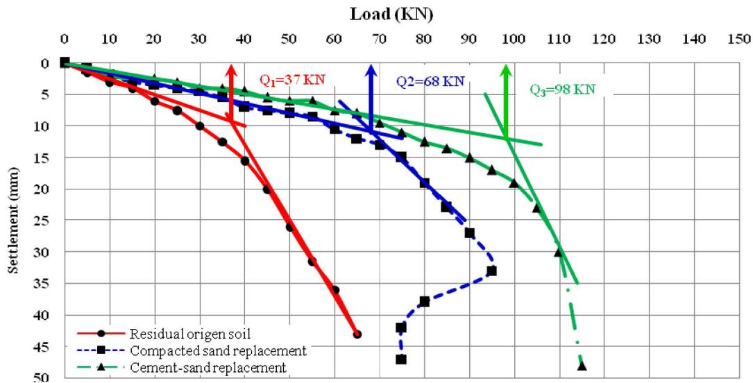
Figure 2. Load settlement response for plate load test.
