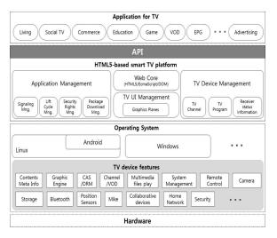
Figure 2. Smart-TV receiver platform architecture
