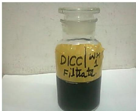
Figure 4: Bio Oil from Water Condenser Collector .
