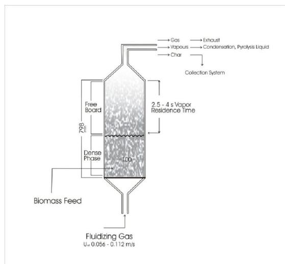
Figure 2: Characteristics of Fluidized Bed Reactor
