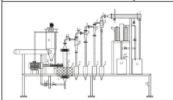
Figure 1: Schematic Diagram of Fast Pyrolysis System: 1. Nitrogen Gas Header 2. Feed Hopper 3. Screw Feeder 4. Fluidized Bed Reactor 5. Reactor Heater 6. Cyclone Separators 7. Char Collectors 8. Hot Filter 9. Water Condenser 10. Dry Ice Condenser 11. Bio Oil Collectors 12. Frame 13. Exhaust Gas 14. Nitrogen Preheater
