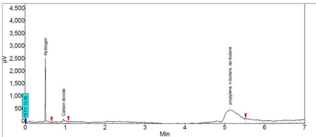
Figure8: Test 2 GC Chromatogram of exhaust gas
