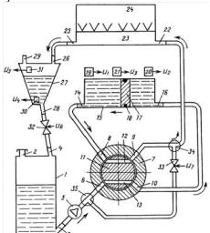
Figure 2. Volumetric flow measurement system of a diesel engine (stable condition 1).
