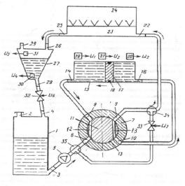
Figure 3. Volumetric flow measurement system of a diesel engine (stable condition 2).
