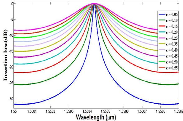
**Fig. 4:** The insertion loss, respect to variation of the coupling coefficient of the add/drop filter system
