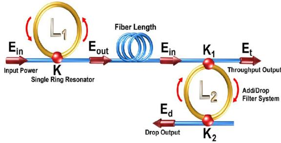
**Fig. 1:** A fiber optic ring resonator is constructed to an add/drop filter system by the couplers
