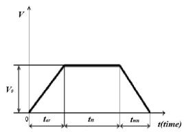
Fig.2 Changes in velocity V drilling tools from time when running in hole.
