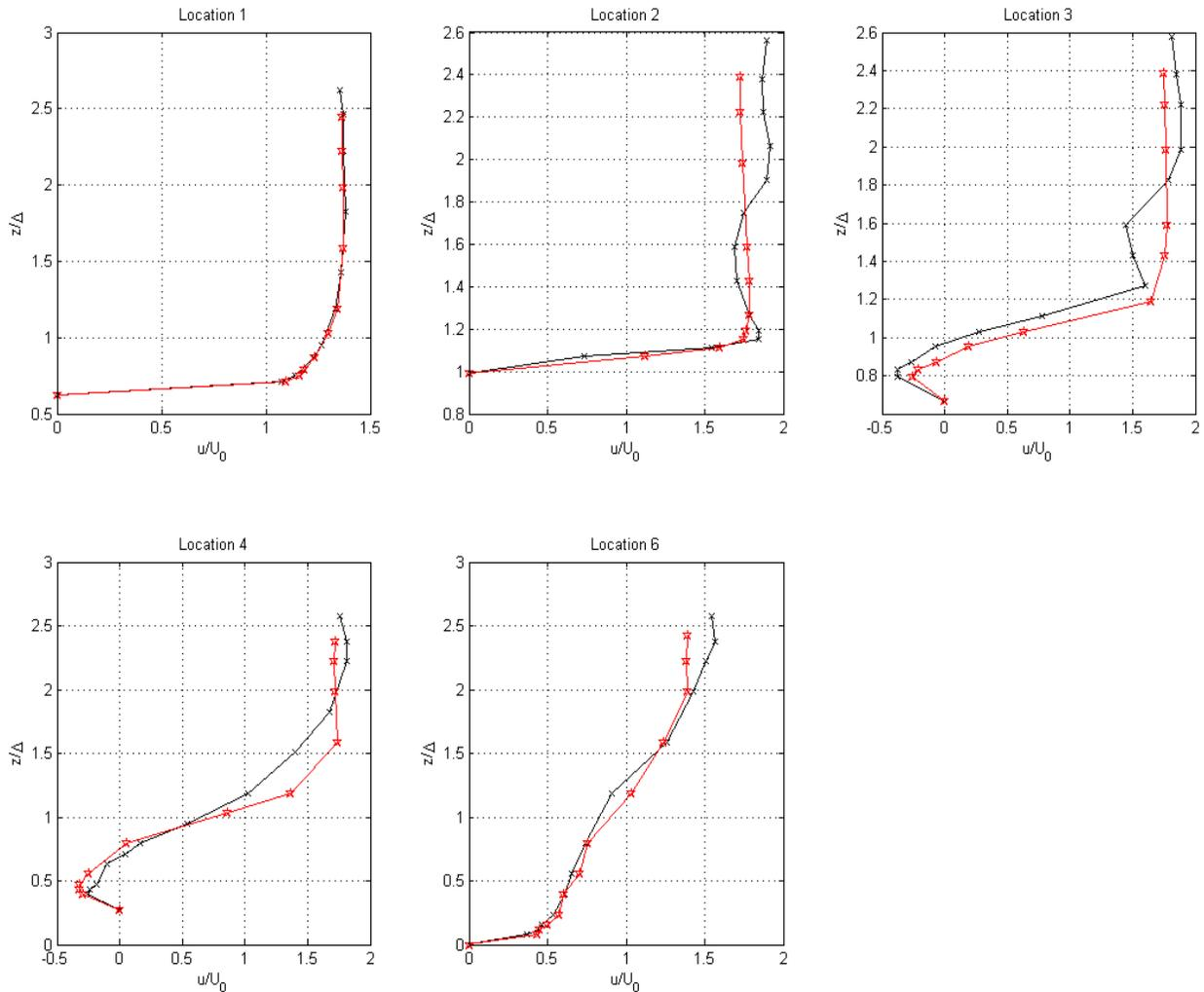
Figure 5(b): Comparison of longitudinal velocity profiles at different locations for the vegetated and non-vegetated weir (\* (red) non-vegetated weir and x (black) vegetated weir  $Q=40$  l/sec).
