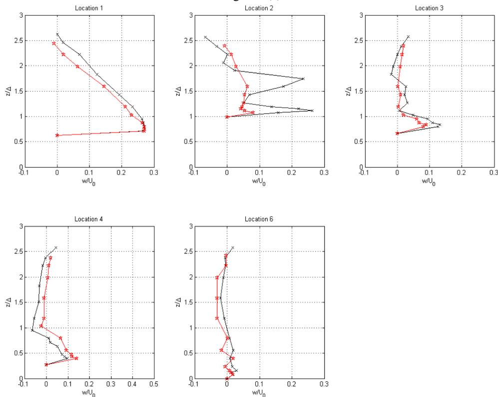
Figure 6 (b): Comparison of vertical velocity profiles at different locations for the vegetated and non-vegetated weir (\* (red) non-vegetated weir and x (black) vegetated weir) (a)  $Q=25$  l/sec, (b)  $Q=40$  l/sec.
