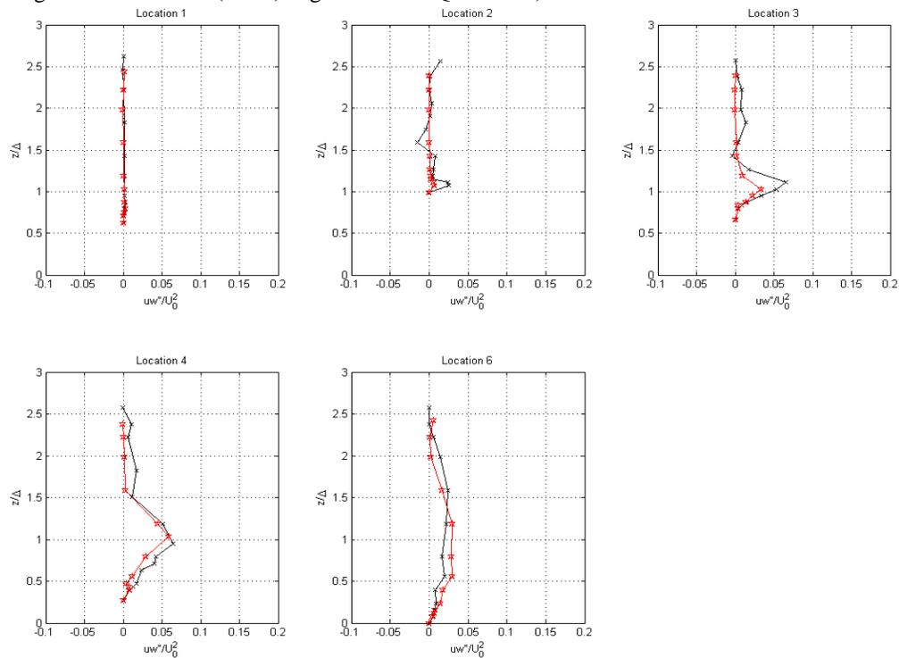
Figure 7(b). Comparison of Reynolds stresses at different locations for the vegetated and non-vegetated weir (\*red) non-vegetated weir and x (black) vegetated weir  $Q=40$  l/sec).
