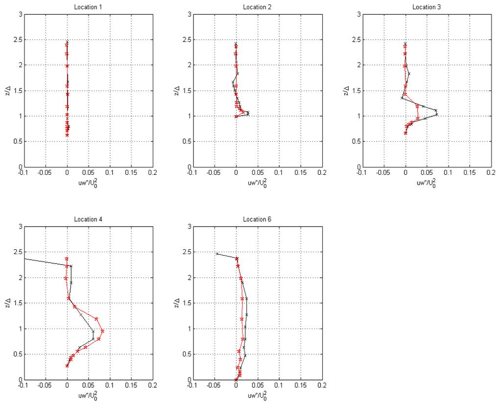
Figure 7(a): Comparison of Reynolds stresses at different locations for the vegetated and non-vegetated weir (\*red) non-vegetated weir and x (black) vegetated weir  $Q=25$  l/sec).
