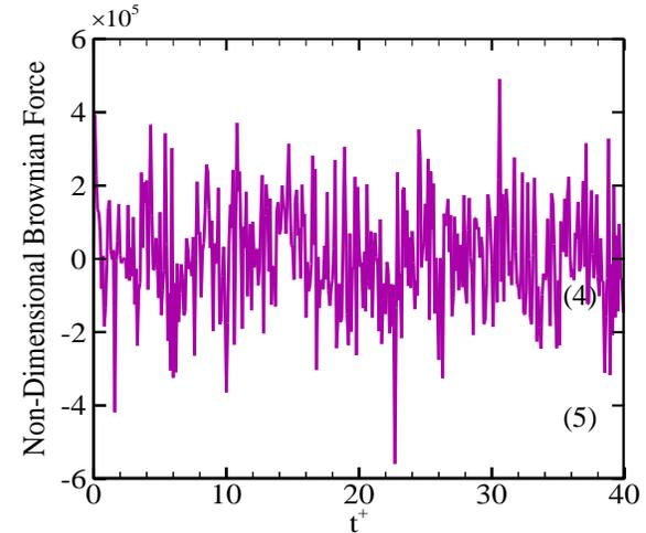
Figure 1: Sample variation of Brownian force for 0.01  $\mu\text{m}$  particle.
