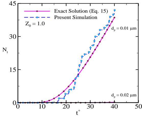
Figure 4. Number of deposited particles with time for different particle diameter and source distance of  $z_0^+ = 1.0$ .
