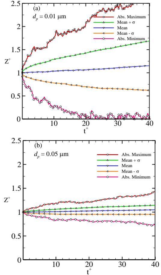
Figure 6. Variation of particle trajectory statics versus time. (a)  $d_p = 0.01\mu\text{m}$ , (b)  $d_p = 0.05\mu\text{m}$ .
