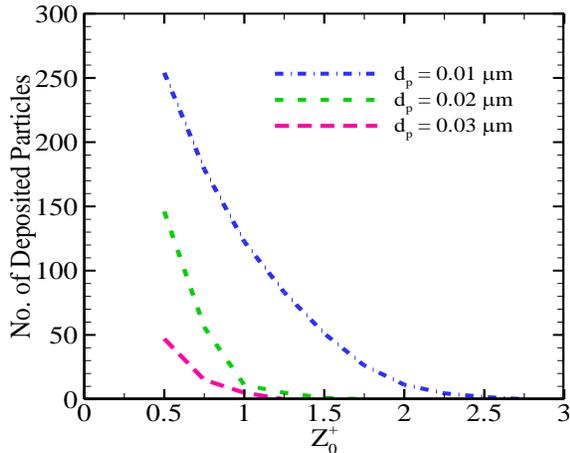
Figure 5. Number of deposited particles with source distance from the wall for different particle diameter and time duration of 100 wall unit.
