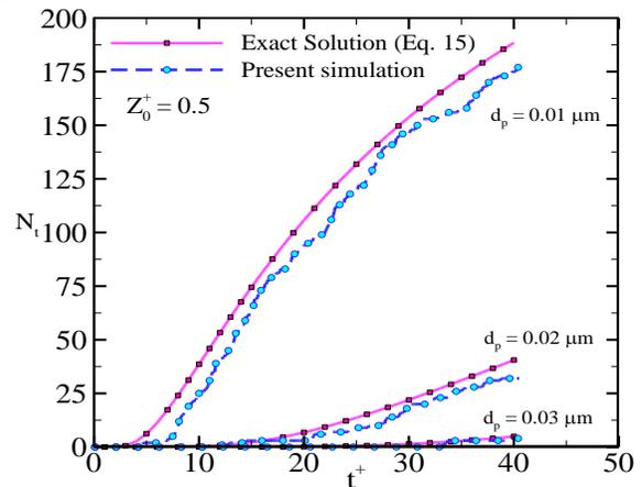
Figure 3. Number of deposited particles with time for different particle diameter and source distance of  $z_0^+ = 0.5$ .
