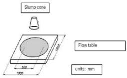
Fig. 2. Slump cone
