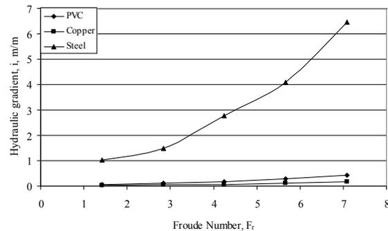
Fig. 9 Hydraulic gradient for 10% of medium sand concentration for different pipes
