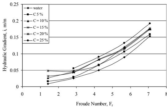
Fig. 7 Hydraulic gradient for medium sand,  $d_{50} = 0.23$  mm through copper pipe for different concentrations
