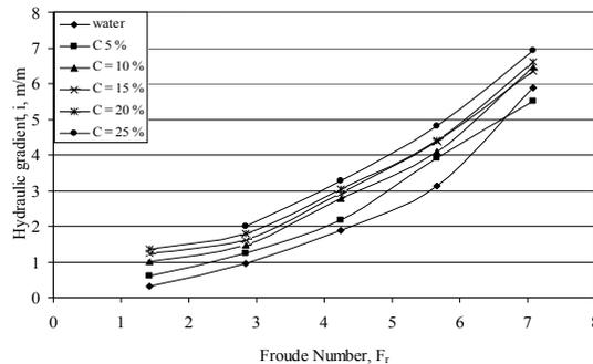
Fig. 8 Hydraulic gradient for medium sand  $d_{50} = 0.23$  mm through steel pipe for different concentrations
