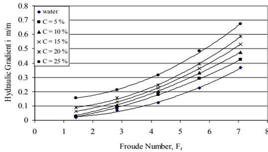
Fig. 3. Hydraulic gradient for finer sand,  $d_{50} = 0.12$  mm through PVC pipe for different concentrations
