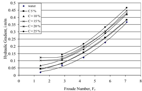
Fig. 5 Hydraulic gradient for medium sand,  $d_{50} = 0.23$  mm through PVC pipe for different concentrations
