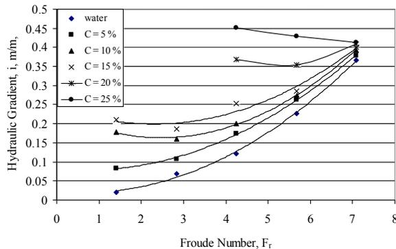
Fig. 4 Hydraulic gradient for coarser sand,  $d_{50} = 0.42$  mm through PVC pipe for different concentrations
