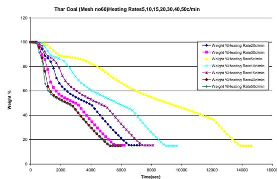
Figure 2: TGA analysis of weight loss (%) as a function of time for different heating rates for Thar Coal of 60 Mesh Size
