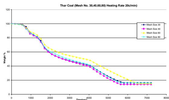
Figure 4: TGA analysis of weight loss (%) as a function of time for different heating rates for Thar Coal of Mesh Size from 30-80
