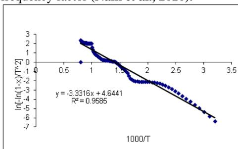
Figure 5: Kinetic plot for a typical heating rate
