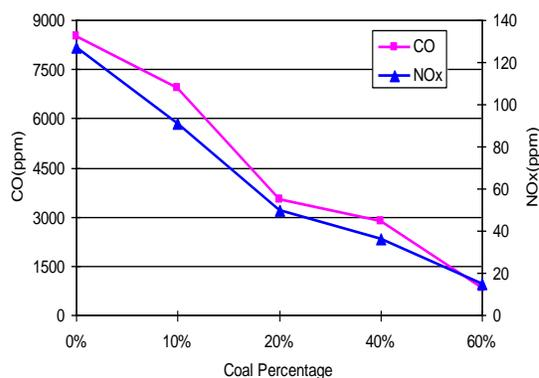
Figure 9 Emission profiles for CO and NO<sub>x</sub> for various coal blending ratios
