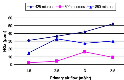
Figure 8 NOx emission for various particle sizes
