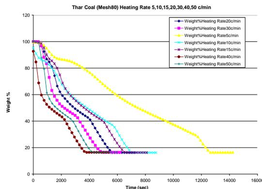
Figure 3: TGA analysis of weight loss (%) as a function of time for different heating rates for Thar Coal of 80 Mesh Size
