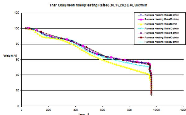
Figure 1: TGA analysis of weight loss (%) for different heating rates for Thar Coal of 60 Mesh Size
