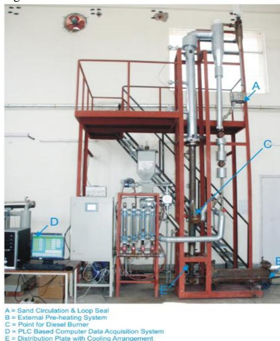
Figure 6: Photograph of CFB test rig
