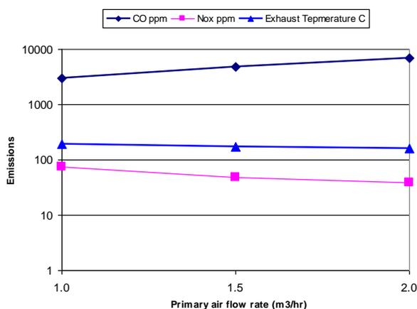
Figure 7: Emission behaviour for particles 212-30 microns
