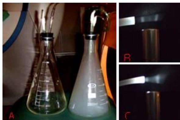
Figure 2: The preliminary results of tests of visualized smoke flow-rate: (A) first burned incense to produce the fume in the erlenmeyer flask for observation (B) At 1mL/s, the shape of visualized smoke was in a columnar shape. (C) At 10 mL/s, the visualized smoke was sprayed.
