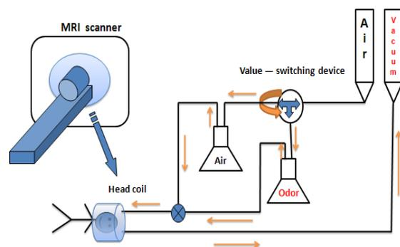
Figure 1: The pipeline design of olfactory experiment.
