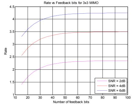
Figure 2 Rate vs feedback bits for 3x3 MIMO system with three different SNR values [14]
