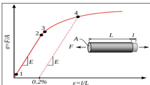
**Figure. (1): Typical yield behavior for non-ferrous alloys, 1: True elastic limit, 2: Proportionality limit, 3: Elastic limit, 4: Offset yield strength (Behiri & Bonfield., 1980)**
