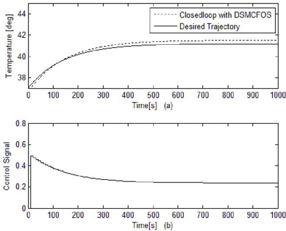
Figure-4 Temperature response for system-I using DSMCFOS (a) Closed loop temperature trajectory and desired trajectory (b) control effort
