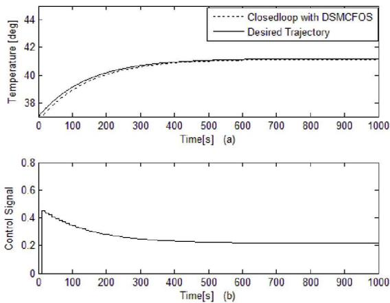
Figure-6 Temperature response for system-III using DSMCFOS (a) Closed loop temperature trajectory and desired trajectory (b) control effort
