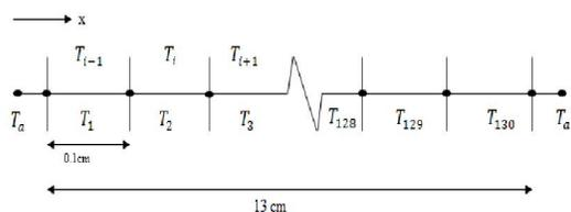
Figure 2 Finite difference nodes in tissue model
