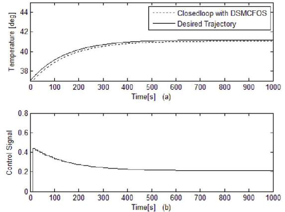
Figure-7 Temperature response for system-IV using DSMCFOS (a) Closed loop temperature trajectory and desired trajectory (b) control effort
