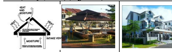
Figure 5. a) Using attics instead of roof insulation, b) Using landscape to moderate air temperature, c) Bigger openings are necessary for cross ventilation
