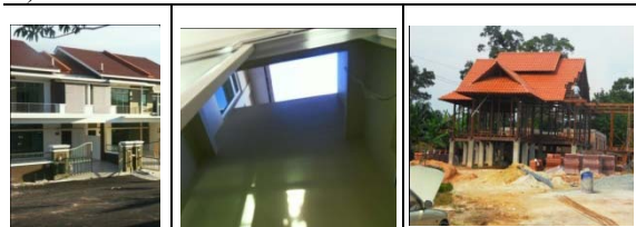
Figure 6. a) Balcony with its aesthetical and functional aspects, b) Ventilation shafts as an alternative to solar chimney, c) Raised floor solves multiple climatic issues such as air-flow and humidity.
