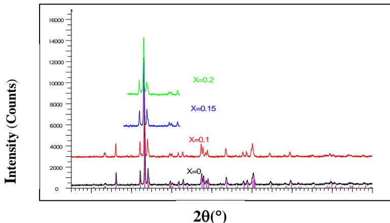
Fig. 1: XRD diffraction pattern of  $\text{Y}_{1-x}\text{Bi}_x\text{FeO}_3$  film for  $x=0, 0.1, 0.15$  and  $0.2$ .
