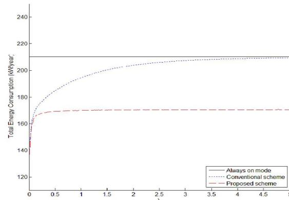
Figure 5. Simulation results of APD and the proposed scheme for variant TV power-on/off rate.
