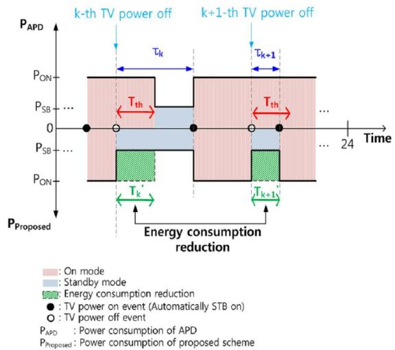
Figure 4. Compare the power consumptions of APD and the proposed scheme.
