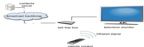
Figure 1. Broadcasting system and set-top-box (STB)
