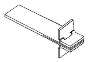
Figure 2. DCB samples for mode I fracture toughness test
