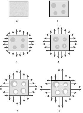
Fig. 4: Mechanisms of Oligomer in increasing the impact resistance of composite samples: The solution of liquid oligomers in the epoxy matrix (0) precipitates into two distinct phase of epoxy and Oligomer spheres (1). Applying the external stress during impact (2) causes the matrix to cavitate (3). The cavities increase by increasing the stress during crack growth (4) and they pin the microcracks that occur during the crack growth (5).
