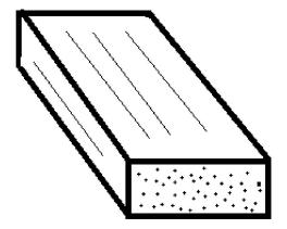
Figure 1. Direction of fibers in the ILSS test samples
