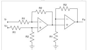
Figure 5- Force/pressure converter
