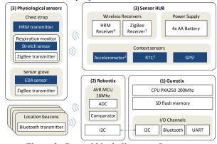
Figure 3- General block diagram of stress measurement system
