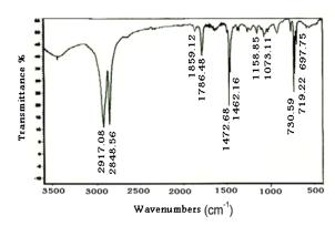
Fig (2): FTIR for Maleated high density polyethylene (MAPE).
