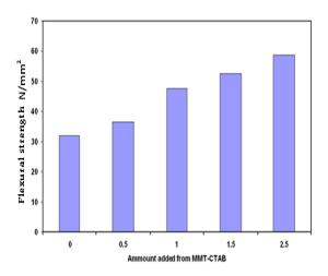
Fig.(9) Effect of added amount of MMT-CTAB on the flexural strength (N/mm²)of the prepared nanocomposites.
