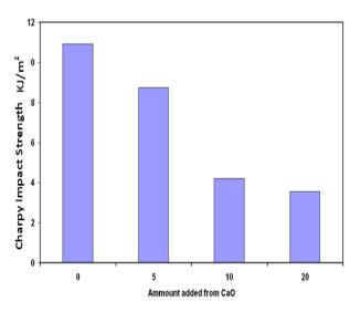
Fig.(12): The change in notched izod impact strength with the amount of CaO loaded with RSF / HDPE composites.
