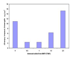
Fig.(11) The change in notched Izod impact strength with the amount of MMT-CTAB increase.
