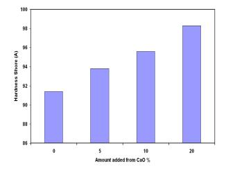
Fig. (14) The change in hardness (shore A) with different amount of CaO.
