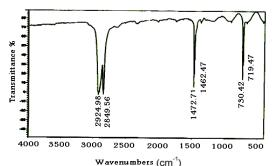
Fig.(1) FTIR for virgin high density polyethylene (HDPE).
