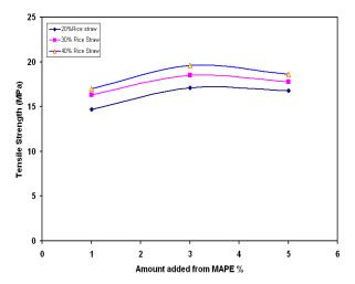
Fig. (3) The change in tensile strength with amounts of coupling agent (MAPE) at different feed ratios
