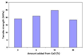
Fig. (7) The relation between Tensile strength (MPa) with different amount of CaO.
