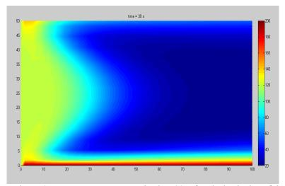
Figure 6. Temperature contour at the time 30s after the beginning of the flow
