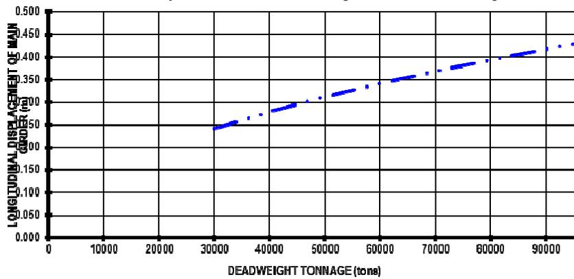
Fig.14. Effect of the Deadweight Tonnage on the Longitudinal Displacements at Midpoint of the Main Girder of the studied models
