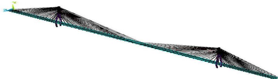
Fig.8. Three-Dimensional Finite Element Model of Tataru Bridge
