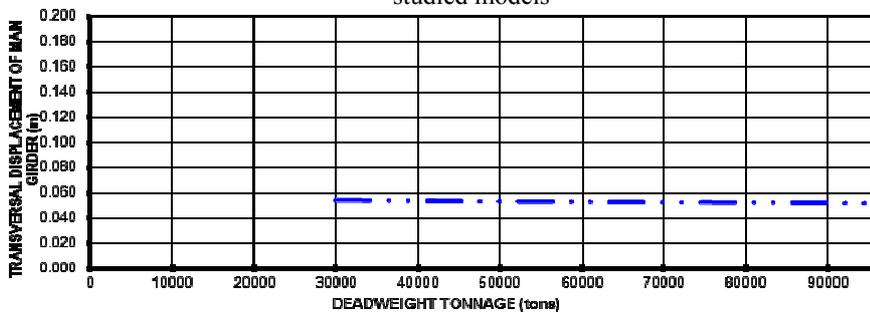
Fig.15. Effect of the Deadweight Tonnage on the Transversal Displacements at Midpoint of the Main Girder of the studied models
