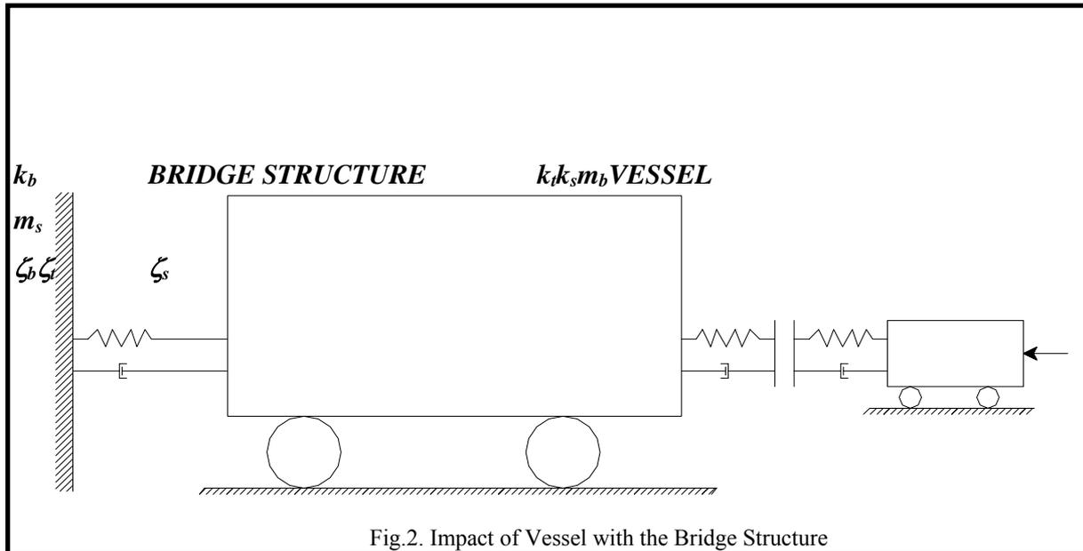
Fig.2. Impact of Vessel with the Bridge Structure
