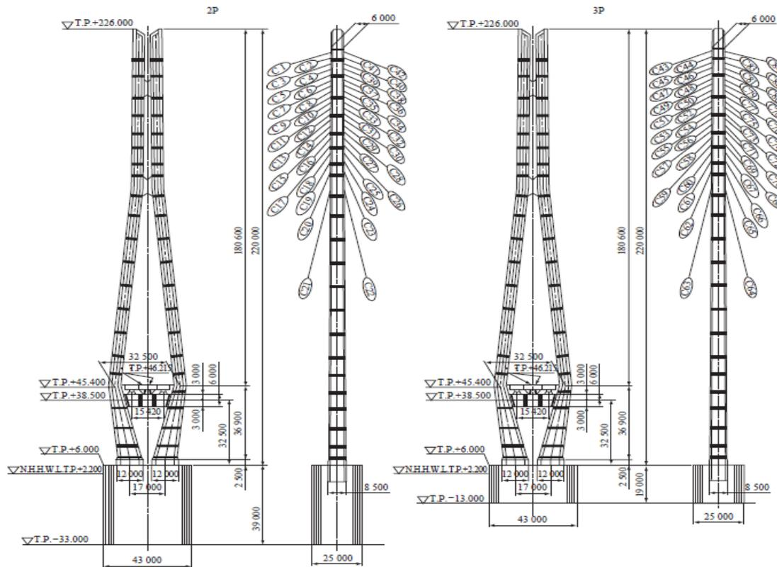
Fig.6. General arrangement (Main Tower)
