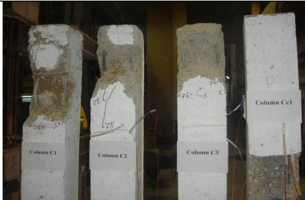
Fig. (8) crack pattern and the shape of failure of c1, c2, c3
