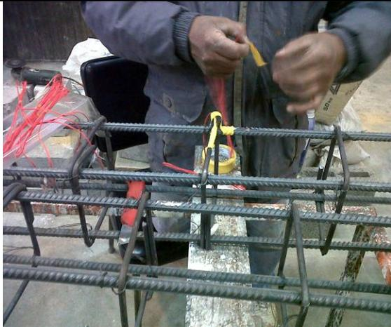
Fig. (3) Fixing electrical strain gages
