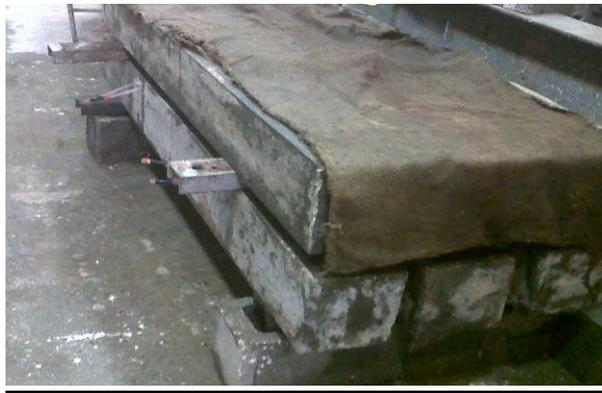
Fig. (5) Specimens curing
