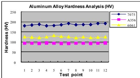
Fig. 4 Aluminum alloy HV hardness test results
