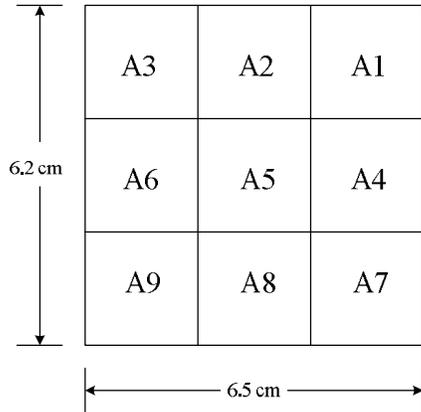
**Figure 2.** The sampling positions of the exposure area applied in the experiments. The diameter is about 62×65 mm in the wedge bottom. The sampling positions of ultrasonic diathermy system is the same as this figure, only the exposure area of ultrasonic diathermy system is about 30×30 mm.
