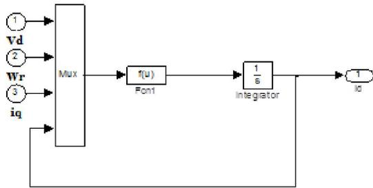
Figure 8 Simulation model of d-axis current
