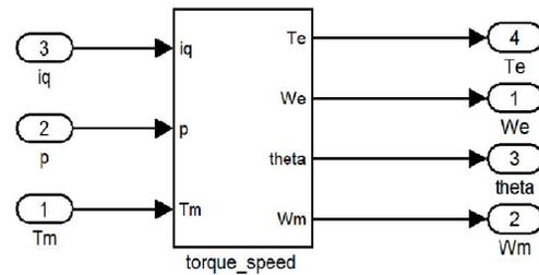
Figure 10 Simulation model of torque and speed
