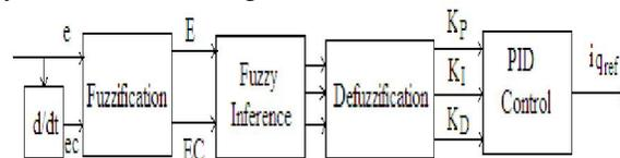
Figure 1 Block diagram of Fuzzy PID controller
