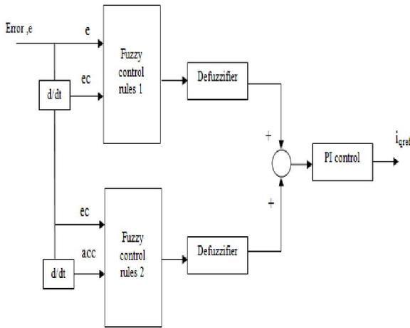
Figure 6 Block diagram of Accelerated Fuzzy PI controller
