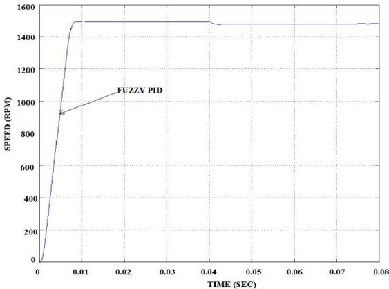
Figure 12 Speed Response of Fuzzy PID Controller
