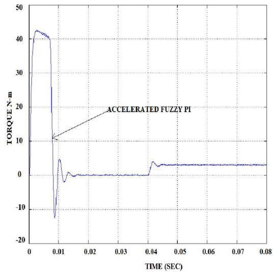
Figure 16 Torque Response of Accelerated Fuzzy PI Controller
