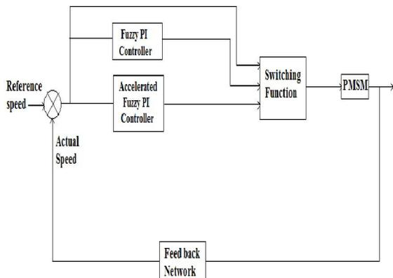
Figure 7 Block diagram of PMSM control system with Intelligent Hybrid Fuzzy controller
