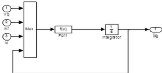
Figure 9 Simulation model of q-axis current
