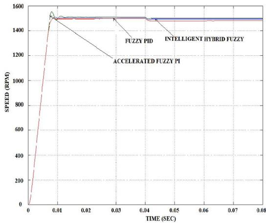
Figure 18 Comparison of Speed for Fuzzy PID, Accelerated Fuzzy PI and Intelligent Hybrid Fuzzy Controllers
