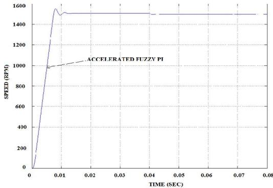
Figure 13 Speed Response of Accelerated Fuzzy PI Controller
