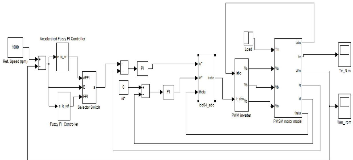
Figure 11 Simulation Model of PMSM Drive System with Intelligent Hybrid Fuzzy Controller
