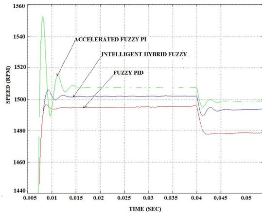
Figure 20 Comparison of Speed drop under load for Fuzzy PID, Accelerated Fuzzy PI and Intelligent Hybrid Fuzzy Controllers
