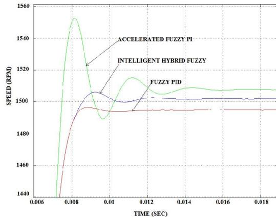
Figure 21 Comparison of overshoot of Speed for Fuzzy PID, Accelerated Fuzzy PI and Intelligent Hybrid Fuzzy Controllers
