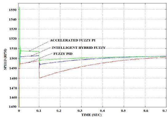
Figure 22 Comparison of Speed under load
