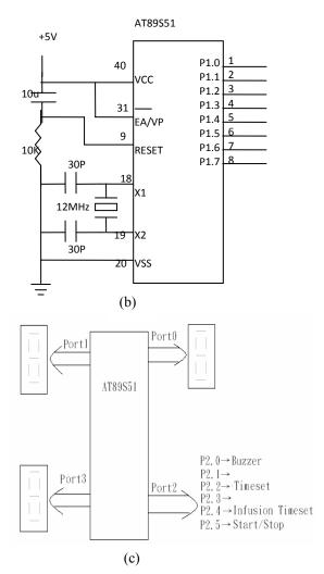
**Figure 1.** (a) AT89S51 pin functions; (b) basic activating circuitry connections; (c) block diagram of loose leaf tea brewing controller.
