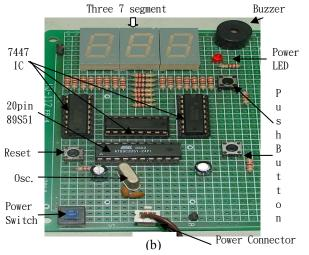
**Figure 3.** Timing controller using (a) 40-pins and (b) 20-pins AT8951.
