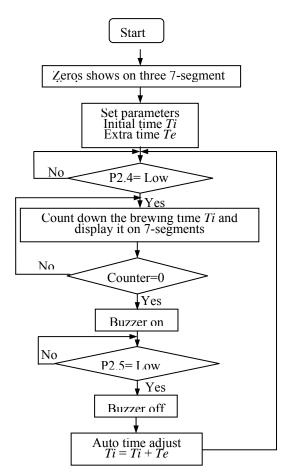
Figure 2. Flow chart of the software control codes.
