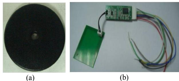
**Figure 2.** (a) RFID tag; (b) reader.
