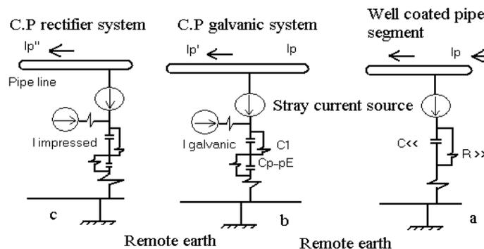
Figure 13: Proposed electrical analogue circuit of the pipe segment-soil system at the cathodic protection process
