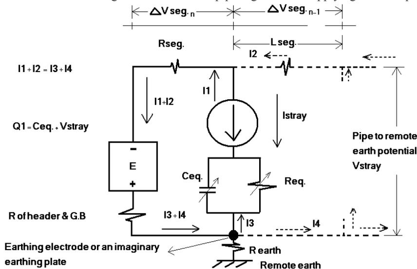
Figure 15b: The final proposed electric circuit diagram of bare pipe segment – soil – earth system with cathodic protection system
