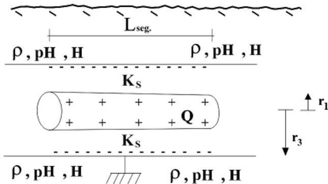
Figure 1: Proposed electrical concept of bare pipe segment with soil medium
