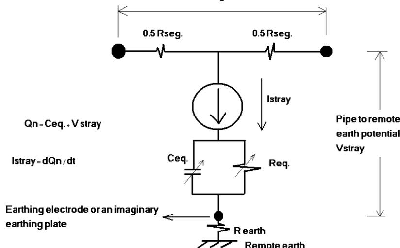
Figure 11: The proposed general electrical analogue circuit of pipe-soil system
