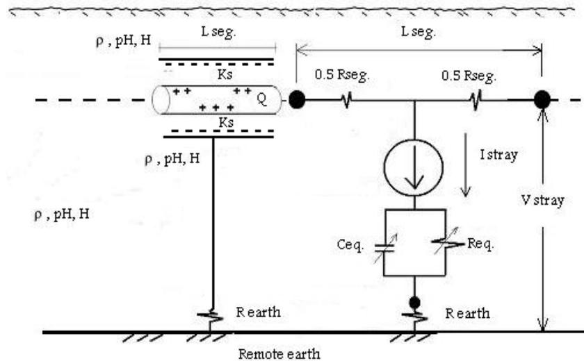
Figure 12: Final proposed electric circuit diagram of bare pipe segment-soil-earth system at natural condition without applying CP system
