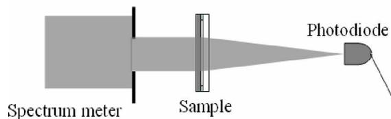
Figure 4. The measurement of transmission spectrum system
