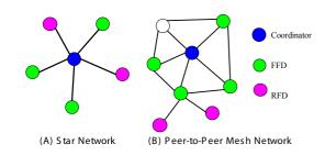
Figure 5. ZigBee Network Topology.
