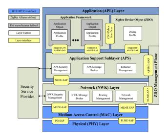
Figure 4. ZigBee stack.
