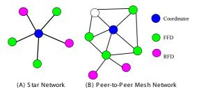
Figure 5. ZigBee Network Topology.
